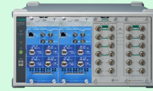
MT8870A Universal Wireless Test Set
